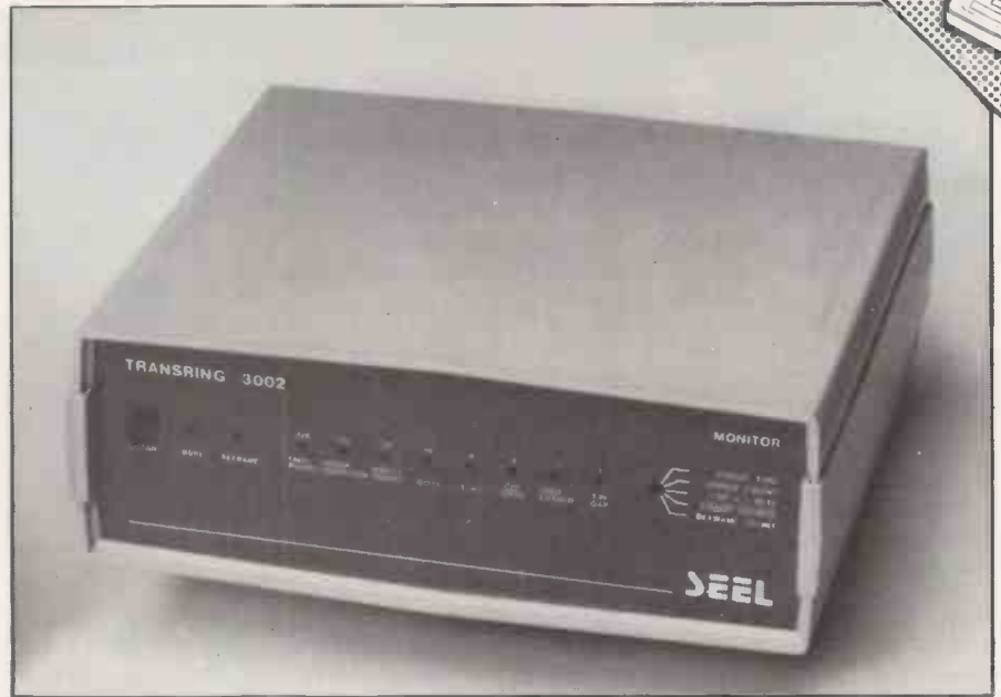
SEEL's Transring employs a Cambridge protocol with twisted-pair or optical-fibre media.
