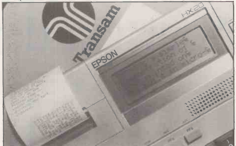
Transam's ITE+ provides 80-column printing on the HX-20's built-in printer.
